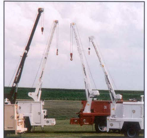
Wide variety of cranes from 2,000 - 14,000 lb. capacity.
