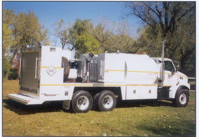
2-Ton Enclosed Reel Lube with Oval Tank & E-Z Pick Electric Crane
