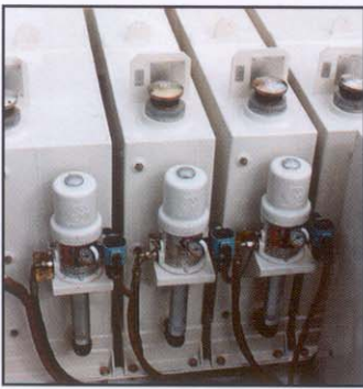
Air Pump Distribution System
